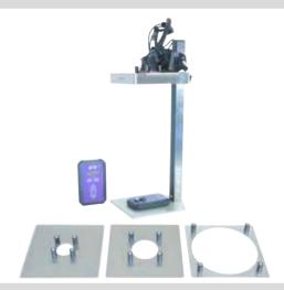
**MEASURING UVG5 UV INTENSITY WITH OLYMPOS** The UVG5 2.0 Spotlight, UVG5 2.0 Midlight and UVG5 2.0 Floodlight can all be measured using the same small size plate.
