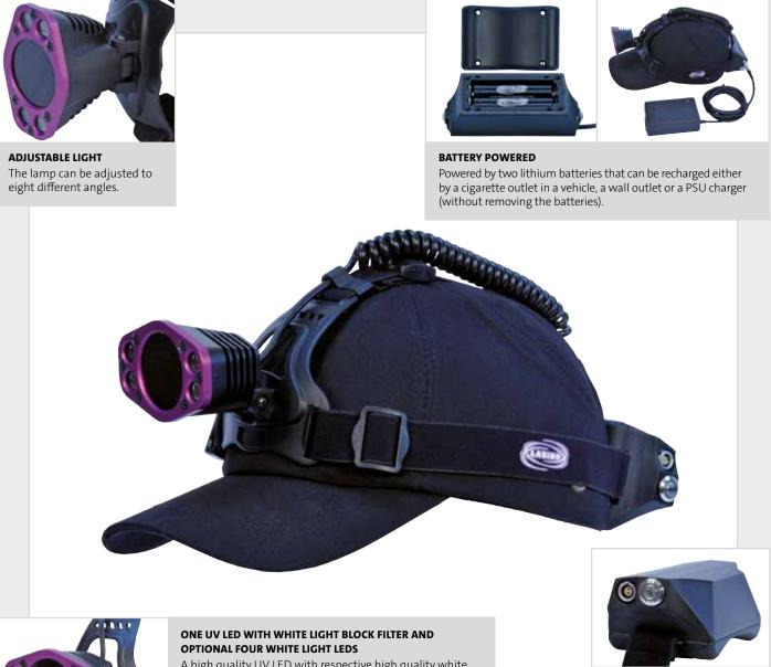
A high quality UV LED with respective high quality white light block filter that does not suffer from solarization. Two different white lights: (a) a strong "search" white light for use in dark and tight spaces such as pipes and tanks and (b) a visual inspection white light.
