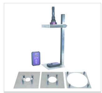
**MEASURING UVG3 2.0 UV INTENSITY WITH OLYMPOS** The UVG3 2.0 Spotlight, UVG3 2.0 Midlight and UVG3 2.0 Floodlight can all be measured using the same small size plate. Olympos measurement stand has part number A542.
