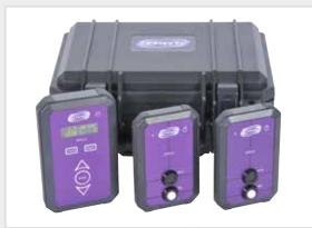
**APOLLO 3.0 DOUBLE KIT PACKAGE INCLUDES:** Reader unit, two sensor units, Calibration certificate, Carrying case.
