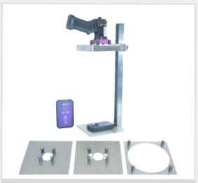
**MEASURING MB 3.0 SERIES UV-A INTENSITY WITH OLYMPOS** Hercules, Zeus, Hermes, Selene and Atlas can all be measured using the same medium size plate.
