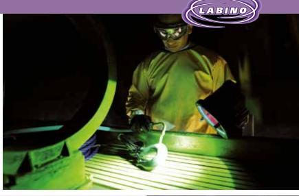
NDI Technician of the 28th Maintenance Squadron performs a magnetic particle inspection to search for any defects on a wire rope hook using a Labino 135 Series UV light at the Ellsworth Air Force Base, S.D.
