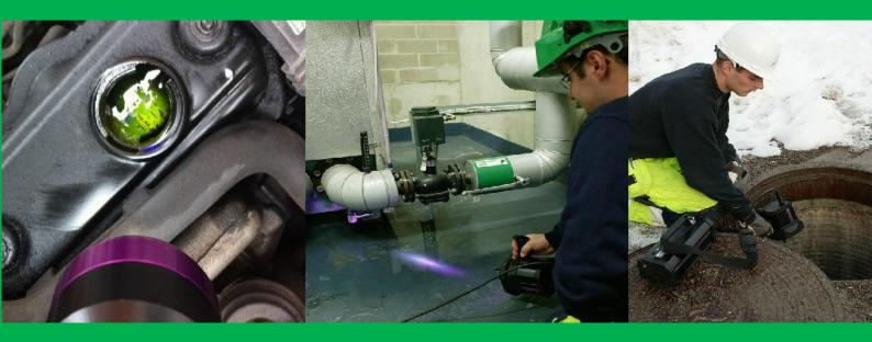
Use Labino Ultra Violet Lamps to detect leakage not visible to the human eye and identify leakage at an early stage.
